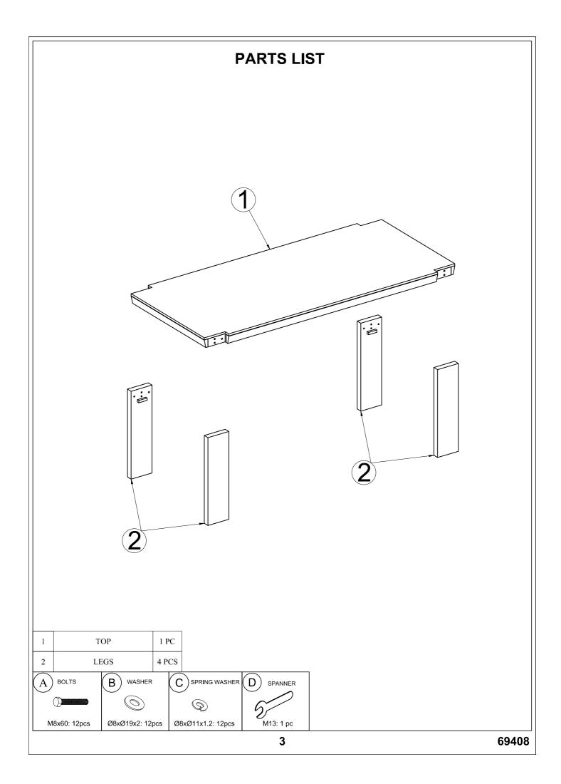
Step 1: Fasten the legs (2) To the top (1) with bolts (A), washer (B), spring washer (C) and using spanner (D)
